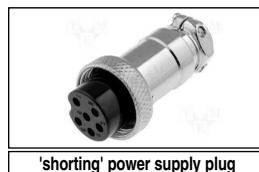
**⚠ Before placing the unit in its chosen location, insert the 'shorting' power supply plug into the PSU socket (7) — see rear panel. Alternatively, you can use the Obelisk PX auxiliary power supply via this socket (see below “Upgrade Options”). If the plug is not inserted in the socket, the preamplifier is completely muted because the circuit is disconnected from the onboard power supply, enabling the connection of the Obelisk PX.**
